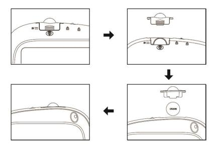
**Battery replacement:** Remove the safety screw and remove the battery holder, remove the battery, insert a new CR 2016 [3V] button cell battery and insert the battery holder back into the slot.
